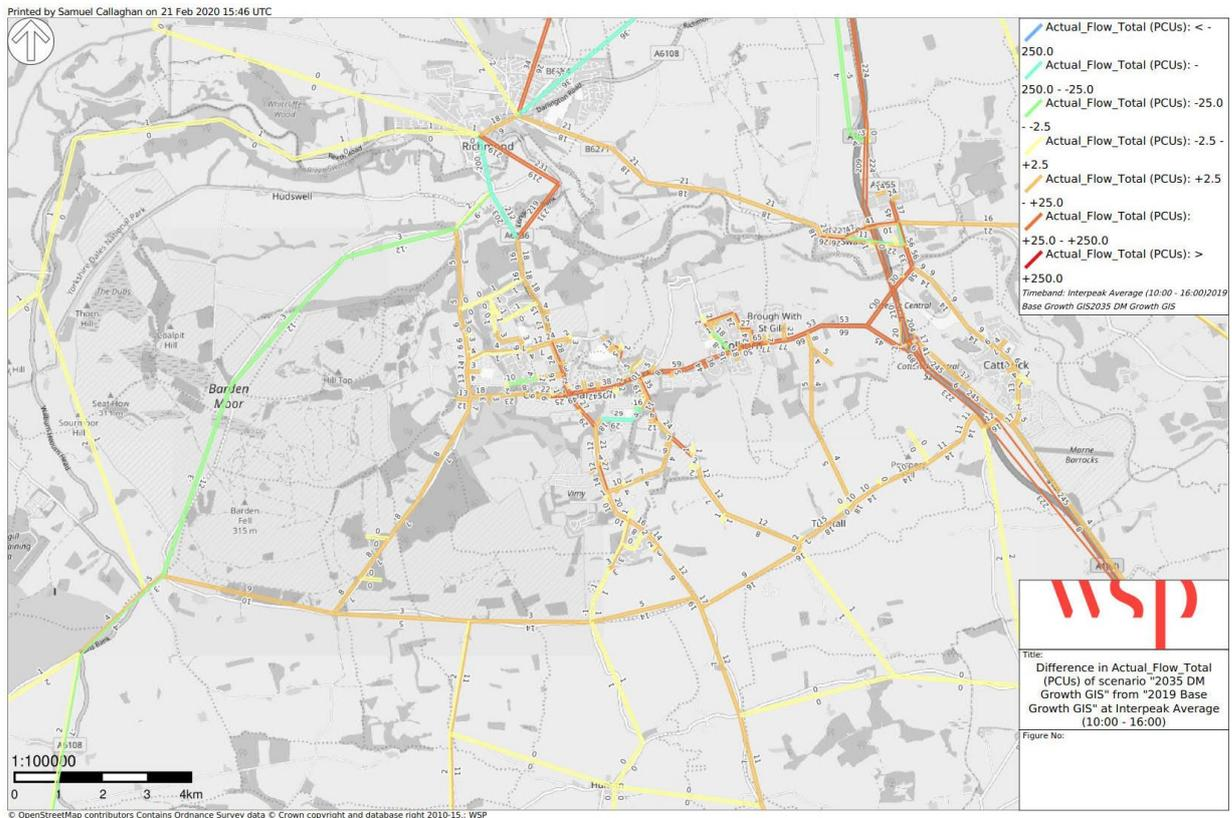
During the AM peak hour, within the simulation area, it can be observed from the above figure that the highest increase in traffic flow is along Catterick Road eastbound and along Richmond Road.
