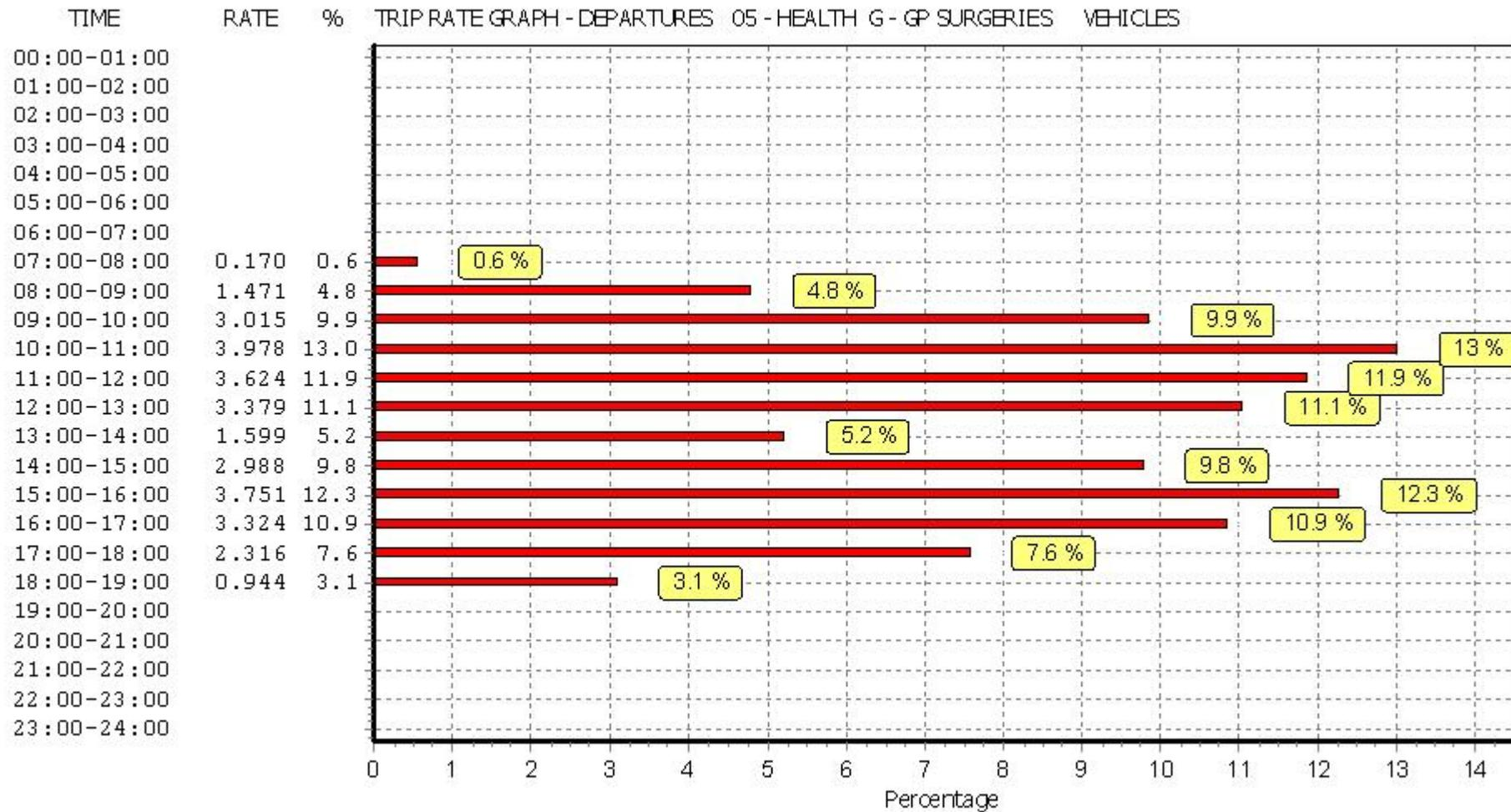
*This graph is a visual representation of the trip rate calculation results screen. The same time periods and trip rates are displayed, but in addition there is an additional column showing the percentage of the total trip rate by individual time period, allowing peak periods to be easily identified through observation. Note that the type of count and the selected direction is shown at the top of the graph.*
