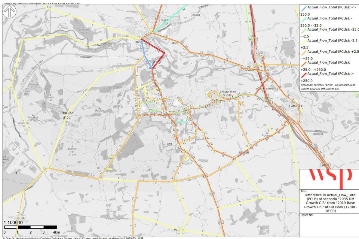
During the PM peak hour, within the simulation area, it can be observed from the above figure that the highest increase in traffic flow is along Richmond Road Scotton Road corridors and
