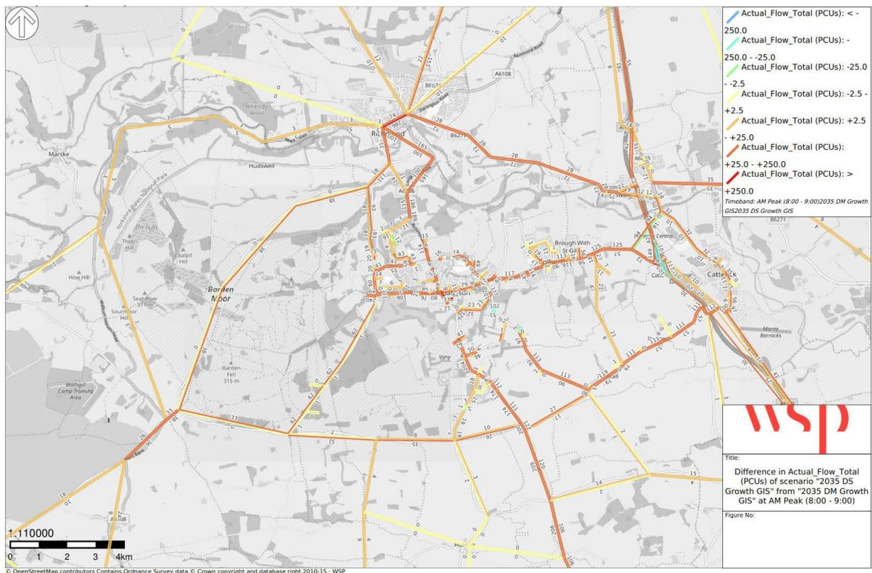
During the AM peak hour, within the simulation area, it can be observed from the above figure that the model predicts considerable increase in traffic flows along all the major roads in the simulation area. This increase can be attributed to the developments included within the DS scenario.
