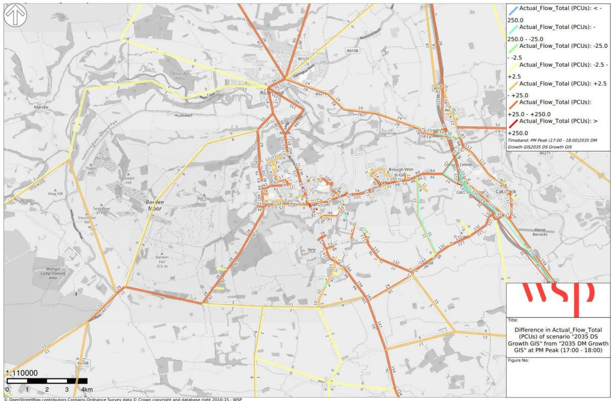
During the PM peak hour, within the simulation area, it can be observed from the above figure that the model predicts considerable increase in traffic flows along all the major roads in the simulation area. This increase can be attributed to the developments included within the DS scenario.
